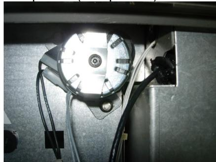
For NON USA appliances the situation is a little more complicated due to the fact that the Factory used an intermediate type of temporary Meteor motoreducer.
