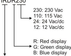
IR: Digital input, RTC and internal buzzer
